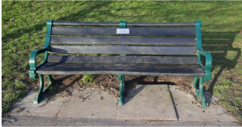
Figure 48 – ‘Brighton bench’ - traditional cast iron ends and legs but with recycled plastic planks.
