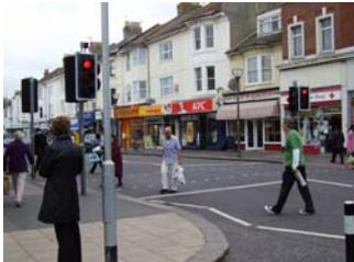
These signalled crossings are used on roads, which have high traffic volumes, high traffic approach speeds or very high pedestrian flows. The time allocated for pedestrian crossing movement is dictated by DETR's guidelines and is based upon the width of the road.
