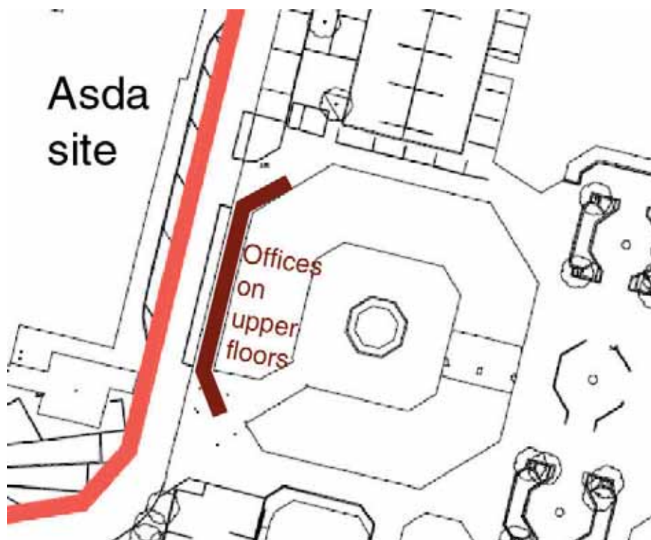
Figure 3 Plan of the Octagon building. The facades highlighted in brown only light offices.
